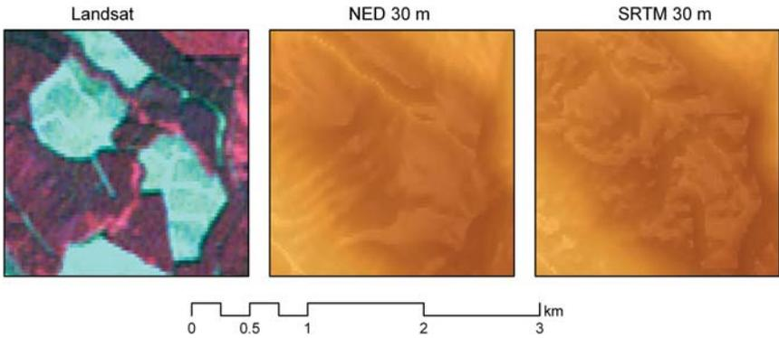
Fig. 9. Comparison of the 30-m NED and SRTM elevation data for a study site in Western Washington near Mount Rainer. Elevation data are shown as shaded relief images. Forest clear cuts are visible on the Landsat image and the boundaries appear as edges in the SRTM data. Such edges increase slope estimates and produce unreliable drainage characteristics.
