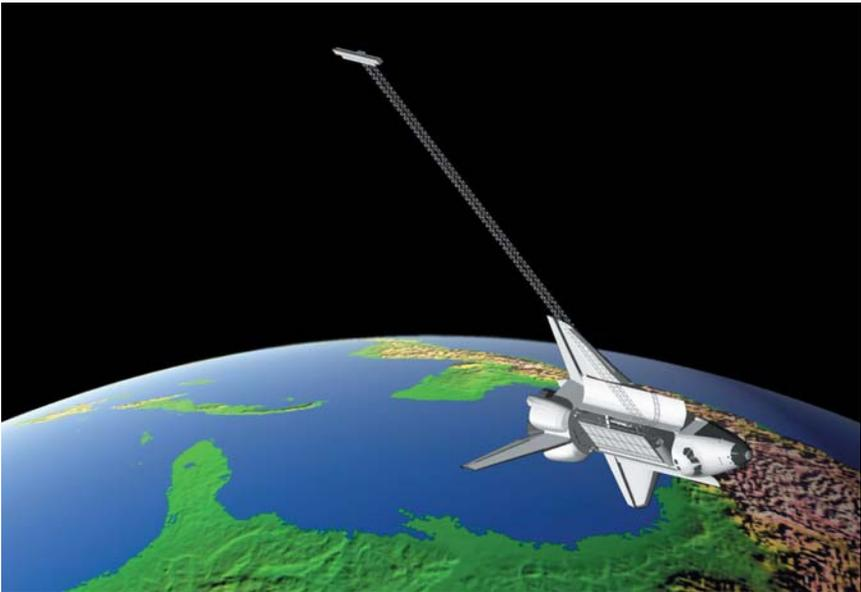
Fig. 3. Computer-generated view of the SRTM mission. The shuttle payload bay contains the main antennas while secondary receive-only antennas are attached to the 60 m long mast. Image courtesy: NASA/JPL.
