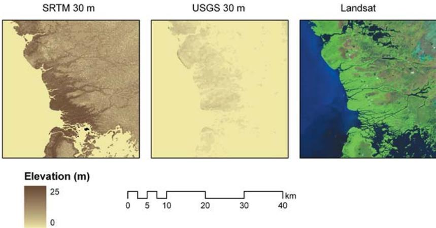
Fig. 12. Comparison of SRTM and USGS DEM for the southwestern portion of the Florida Everglades. The USGS DEM is a bare-earth DEM derived by the interpolation of a large number of ground control points. The SRTM elevation values are clearly much higher and reflect the mangrove forest in this area. Subtracting the bare-earth DEM from the SRTM DEM provides an initial estimate of mangrove height, but requires adjustment for vertical bias, as well as calibration with field surveys or airborne LIDAR.
