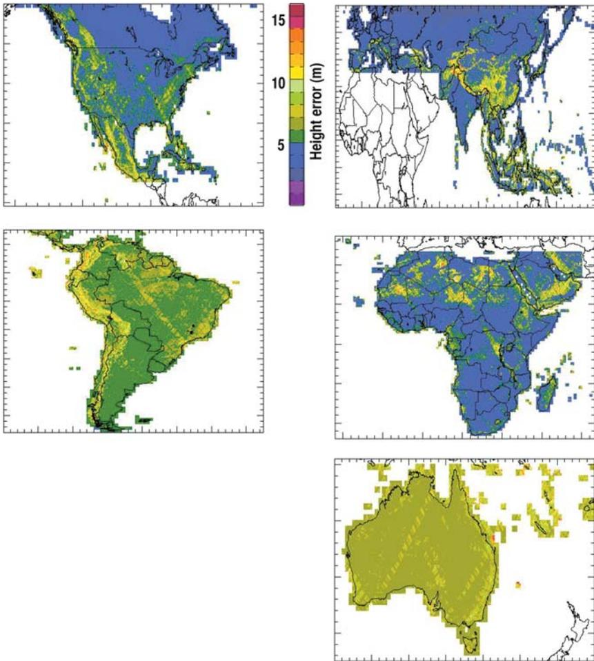
Fig. 5. Absolute vertical error of STRM data by continent. The 90th percentiles are: 5.6 m for Africa, 6.0 m for Australia, 6.2 m for Eurasia, 9.0 for North America and 6.2 for South America. Image courtesy: NASA/JPL.
