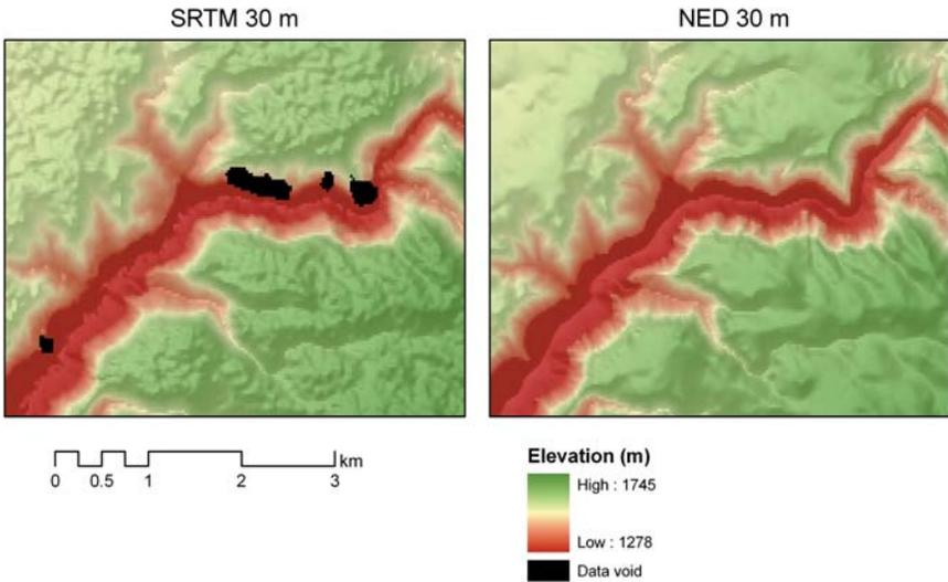
Fig. 7. Hillshaded elevation model of a small part of the Grand Canyon in the United States. SRTM elevation data are shown on the left and NED elevation data are shown on the right. The SRTM data reveal a number of typical voids (shown in black) on steep slopes.
