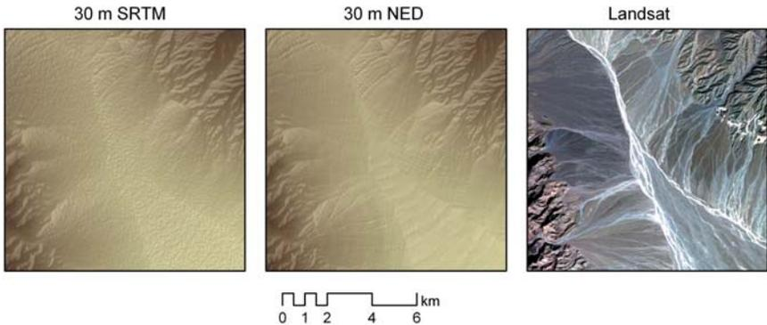
Fig. 6. Hillshaded elevation model of a small part of Death Valley in the United States. The SRTM data reveal a substantial amount of speckle noise. The NED elevation model is much smoother, although some of the artifacts of interpolation from contours are visible.
