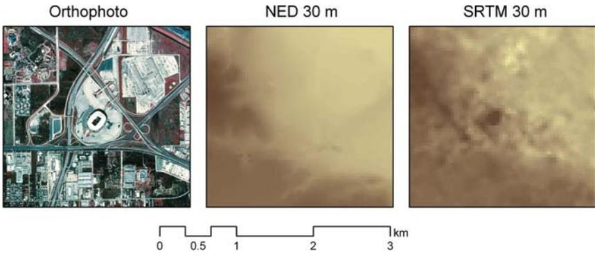
Fig. 10. Comparison of the 30-m NED and SRTM elevation data for Texas Stadium in Dallas, TX, USA. Elevation data are shown as shaded relief images. While the structure is clearly identifiable in the SRTM elevation model, the bare-earth NED elevation model does not reveal the structure.
