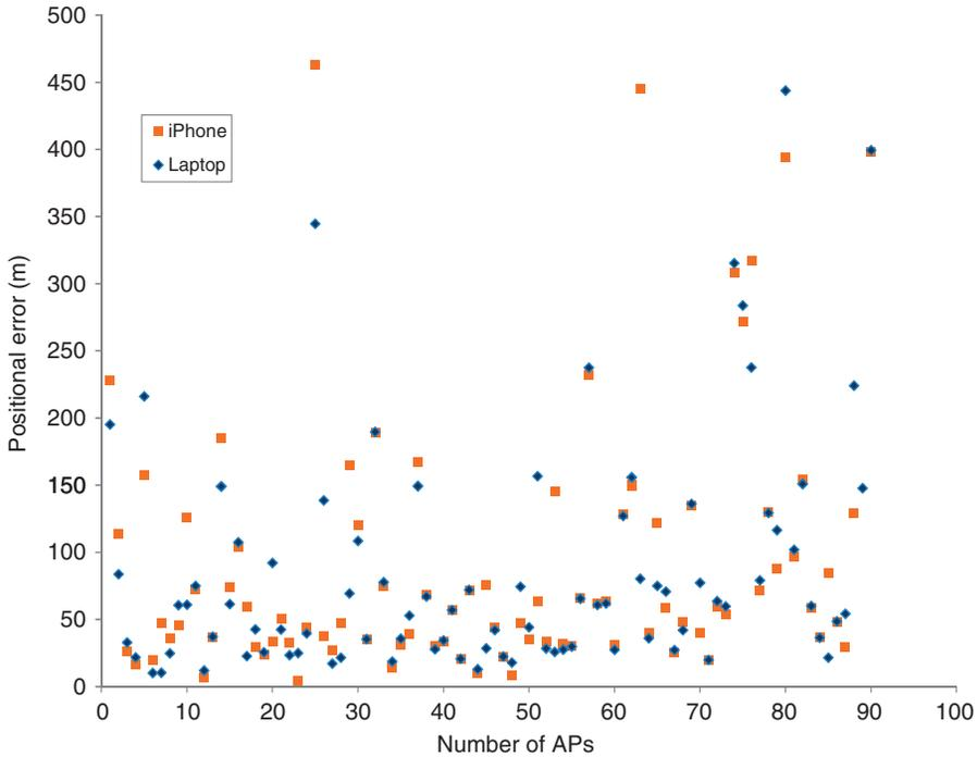
Figure 3. Relationship between the number of WiFi APs and positional error (m) on two mobile devices.
