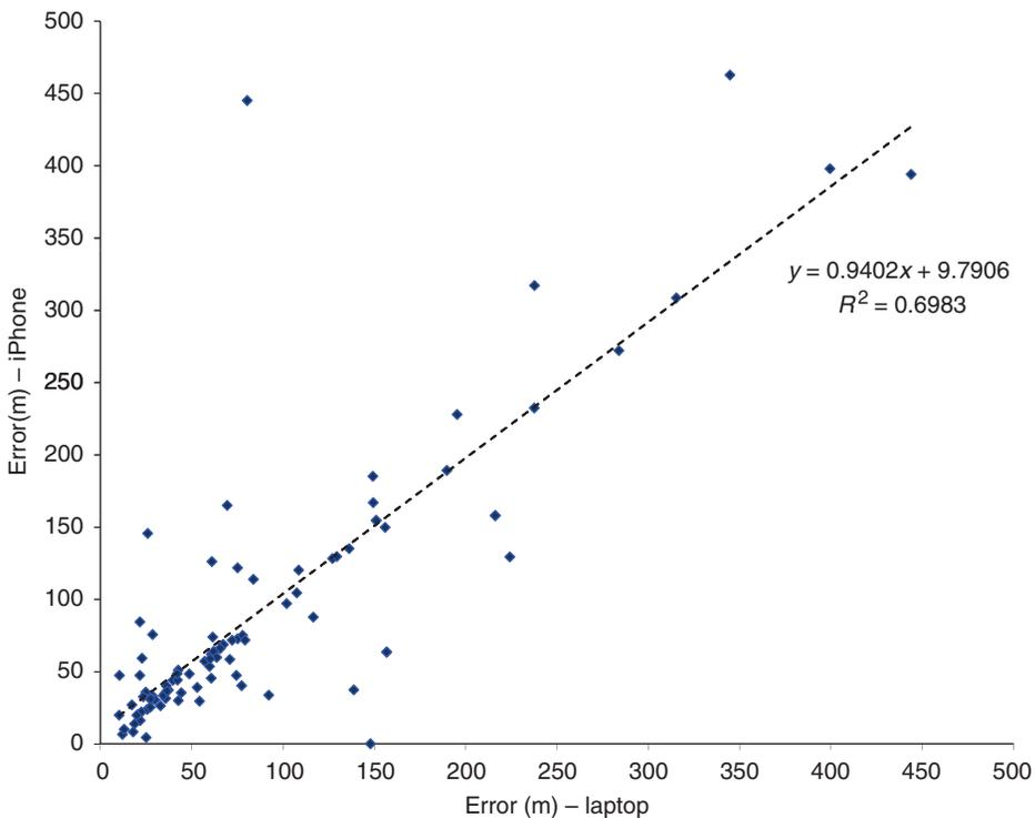
Figure 1. Correlation between the positional error of WiFi positioning on two mobile devices.
