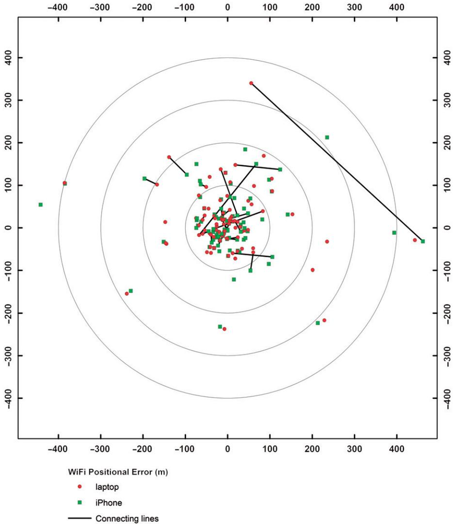
Figure 4. Positional error of WiFi positioning (m) relative to reference location.
